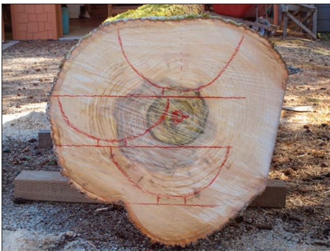
1. Three possible bowl orientations are drawn on the butt of this log. Note that all options exclude the pith, the source of much of the tension in a tree.
